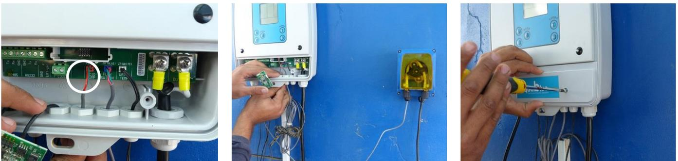
6. Wire the electrical cable of the acid pump to the main power source in the machine room (240V) parallel to the circulation pump. **This must be performed by a licensed electrician!**
