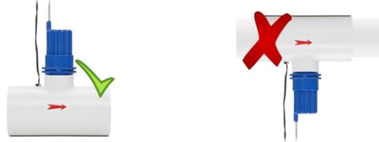
3. **Make sure that the arrow at the top of the flow sensor points in direction of the flow and that no glue or pipe cleaner touches the paddle inside the sensor as it may cause it to jam.** Double check that the flow sensor operates properly by reducing the flow for five seconds and checking if the low flow indicator on the control box lights.
