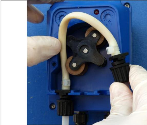
Gently insert the tube back into place making sure the black bases of the tubes are tightly in their slots in the casing.
