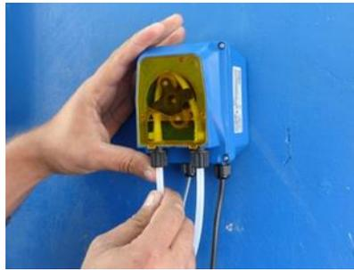
13. Thread the other end of suction tube through the lid of the acid container and attach to it the weight and foot filter.
